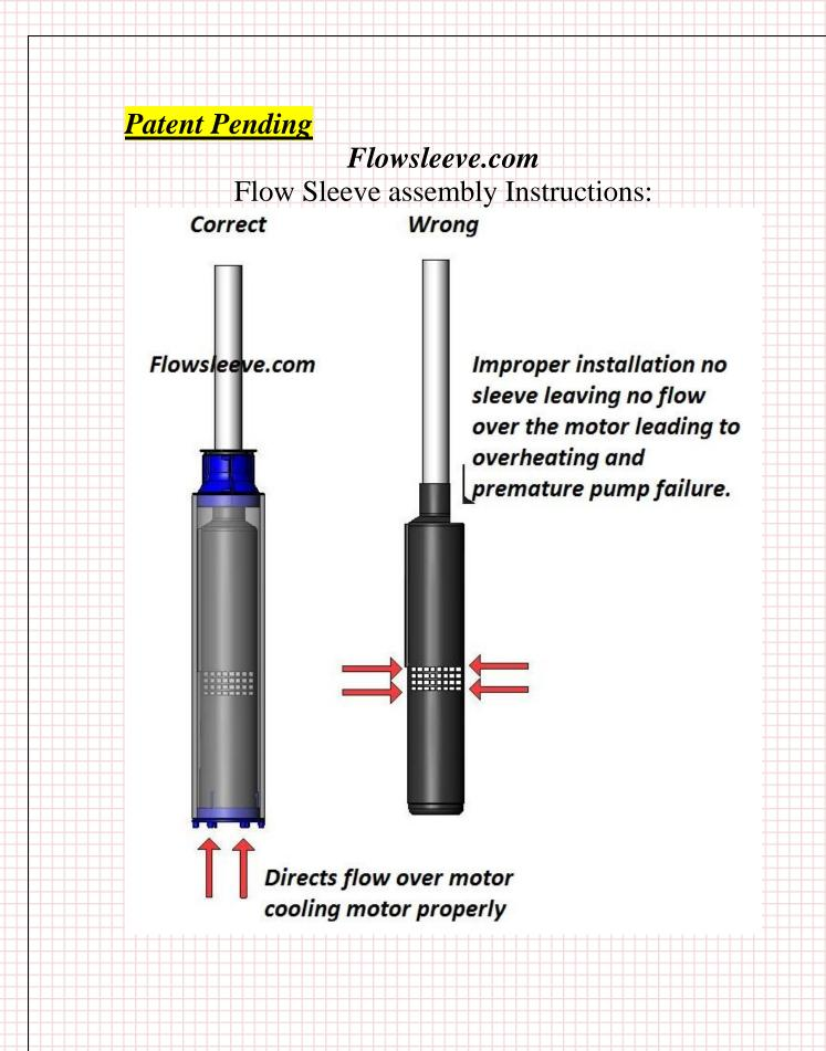
1. Assemble Pump motor, and splices as per manufacture Instructions.
