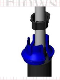
5. Hold part C up to the bottom of the motor and measure between Part C and A&B. Cut length of pipe to this measurement.
