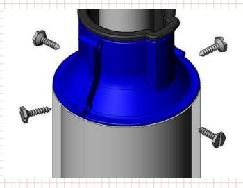
Slip Part D into bottom of pipe centering motor in place. Secure with 4 each Stainless steel screws.
